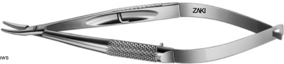
ZI-32315 BARRAQUER Needle Holder curved, without lock 8 mm standard jaws 1.2x0.8 mm tips original model with longitudinal groove handle diameter 10 mm overall length 130 mm
